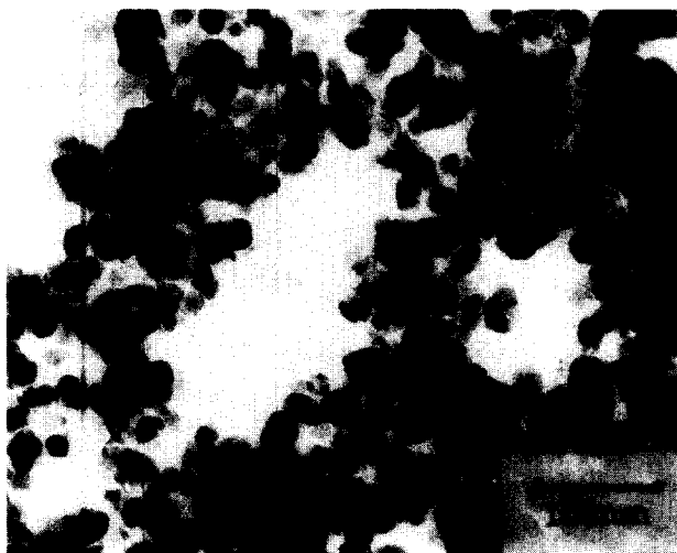
Fig. 3. TEM micrograph of Cu particles after milling with NaCl added in the starting material and subsequently washed.
